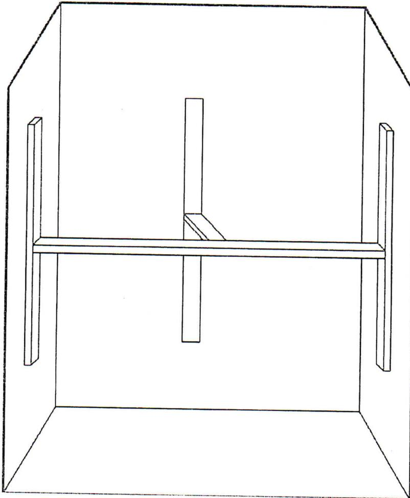
After the MPL 100% Silicone adhesive has set-up, remove bracing. Silicone all the joints where marble touches marble or shower pan/tub, with MPL Color Match 100% silicone. Caulk the areas where marble touches drywall, or other substrate material, with a latex paintable caulk.
