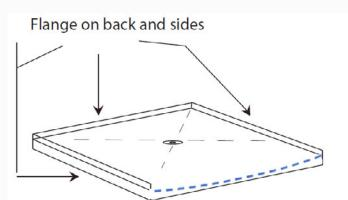
With the built-in slope to drain, the front edge will have a slight 'smile'.
