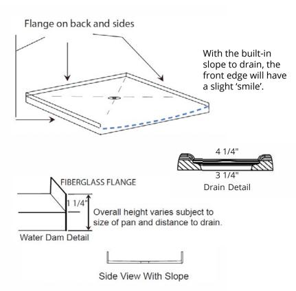
It is required for ADA Compliance that the finish floor is 'floated' to meet the height and 'smile' of pan's front edge.
