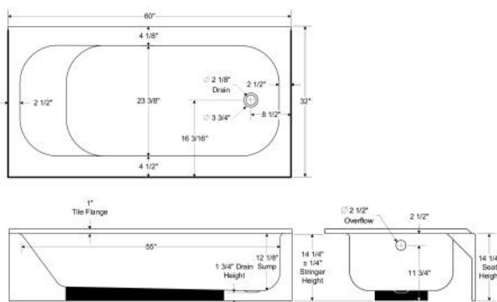
All dimensions are approximate. Structure measurements must be verified against the unit to ensure proper fit. Please see the detailed technical drawing for additional measurements.
