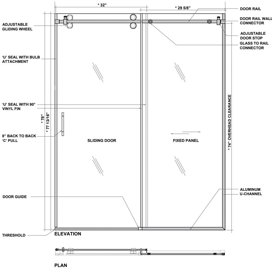
\*NOTE: Nominal Sizes. These measurements are based on a standard 60"x78" enclosure. Heights and Widths are variable and can be ordered to fit specific project requirements.
